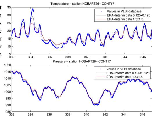
Figure 3: Pressure (in mbar) and temperature (in Celsius degrees) time series for the station HOBART26 during CONT17 from three different sources.
