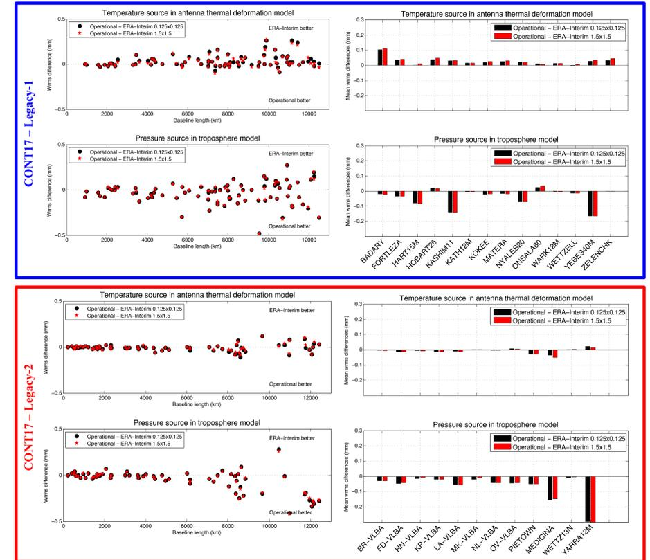
Figure 4: Differences in baseline repeatability (left) and in station repeatability (right) between an operational solution and a solution using the temperature from ERA-Interim in the antenna thermal deformation model (top), and the pressure from ERA-Interim in the troposphere model (bottom). Legacy-1 stations in blue box. Legacy-2 stations in red box.
