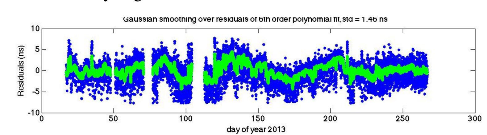
Random walk of the hydrogen maser time at NGSLR over 8 months after removing a polynomial fit, mostly a constant offset and a linear frequency aging trend.
