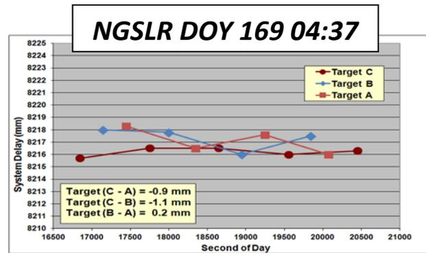
**Satellite Data Analysis:** Satellite data is analyzed using POLYQUICK software [[https://ils.gsfc.nasa.gov/network/system\\_performance/polyquick.html](https://ils.gsfc.nasa.gov/network/system_performance/polyquick.html)] which directly compares all simultaneous normal point data. The satellite data is used to detect biases between the two systems.
