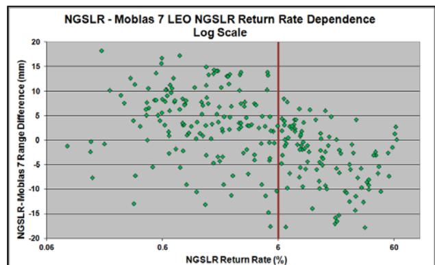
return rates (< 6%) is 4.0 mm, while at higher return rates (>6%) is -3.4 mm. The higher signal strength is producing multi-photon returns causing the single photon detector to bias the data short.
