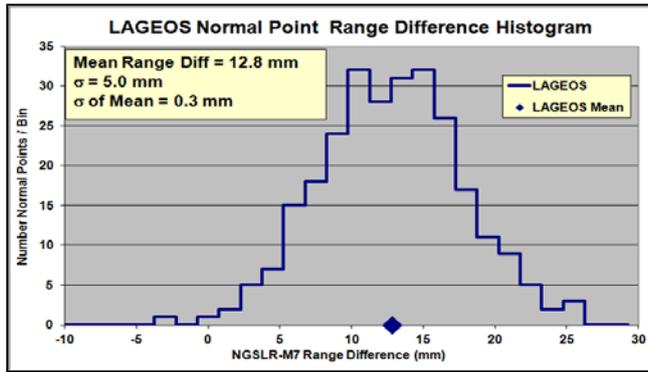
This histogram shows a symmetric distribution of the NGSLR / MOBLAS-7 collocated LAGEOS normal point range differences. The distribution of the normal point differences is consistent with previous MOBLAS-7 collocations with other systems, and the mean range difference of 12.8 mm is in agreement with theoretical values.
