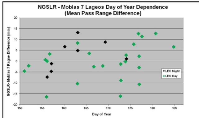
The following charts, showing normal point range differences, are designed to find potential dependencies in satellite return rate. The NGSLR Return Rate (log scale) LAGEOS dependency plot displays no significant trends. The LEO range differences are biased at higher return rates as expected when comparing single and multi-photon returns. The mean range difference at lower
