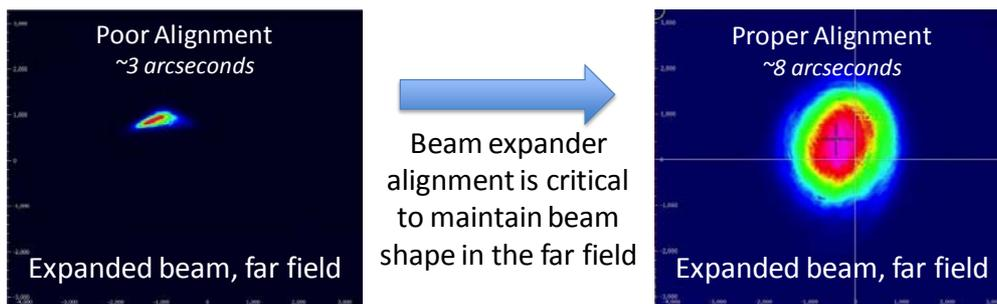
Figure 6 – Using the Beam Profiler to verify the alignment of the Beam Expander
