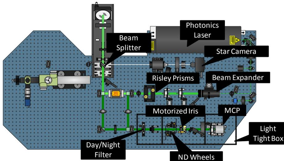
Figure 4: Layout of the Third Generation Optical Bench
