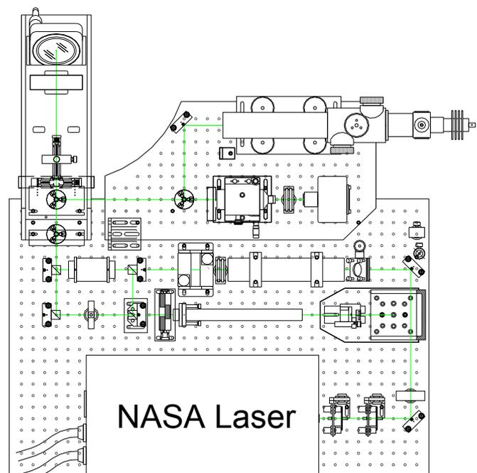
Figure 2: Layout of the Second Generation Optical Bench
