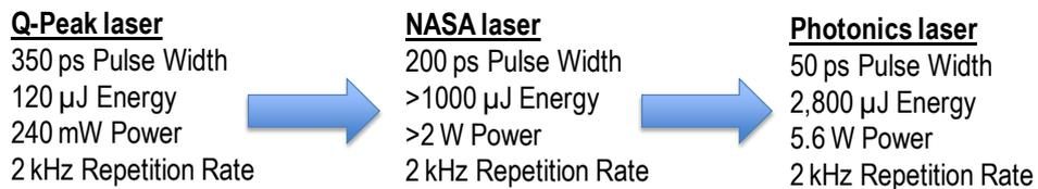
Figure 3: Progression of Laser Upgrades
