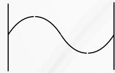
Wavelength is the length of one complete cycle of an electromagnetic wave.
