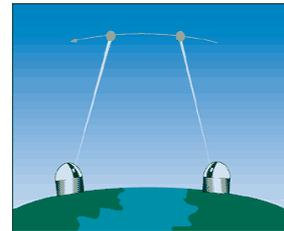
**VLBI:** Radio telescopes equipped with X/S wideband receivers record signals from quasars to measure difference in signal arrival times
