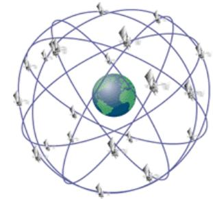
**GNSS:** Satellites (GPS-U.S., Russia-GLONASS, EU-Galileo) equipped with precise clocks transmitting messages such as ephemeris, clock offsets, etc. to ground (and space-based) receivers to measure station to satellite pseudo-range, phase delay
