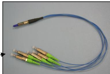
Each fiber couples to a separate Si APD detector
