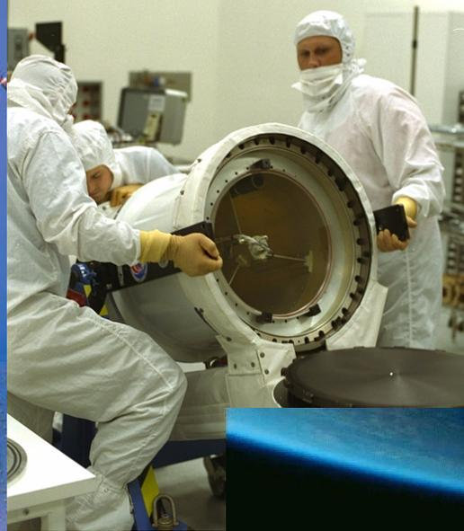
Laser Altimeter Canister integration into HH canister prior to SLA-01 Mission
