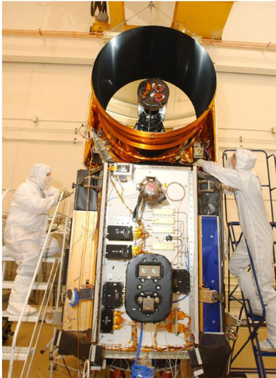
GLAS being integrated onto the spacecraft at the Ball Aerospace in 2002
