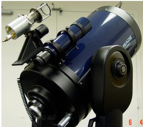
The GLAS EM detector and aft optics piggy backed on a Meade 10" telescope. A diffuser was placed in front of the detector to attenuate the signal by ~1000 and widen the field of view to +/-3° FWHM.
