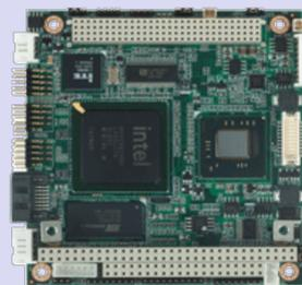
The test bed consists of three PCM-3362Z2-1GS6A1E boards. The PCM board is a PC/104-Plus that has an Intel Atom N450 Processor, 224 MB shared memory, two serial ports for communication, and 8-bit general purpose Input/Output. These boards are three components that HyMAS is divided into.
