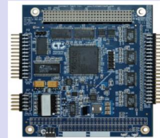
The Xtreme I/O ADC-DAC DAG003. Connect Tech Inc designed the Xtreme I/O analog and digital peripheral board. The Xtreme I/O board has 16 differential channels of analog input with 16-bit resolution. The ADC is created for the form factor of a PC/104-Plus bus and a sampling rate of 100,000 samples per second
