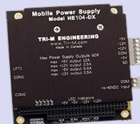
Four HE104+DX power supplies are needed to give power to each board and also reduce some radio frequency noise that would interfere with receiving accurate data. The HE104+DX is a high performance DC-to-DC converter that supplies +3.3V, +5V, +12V and -12V outputs to the PC/104-Plus bus.
