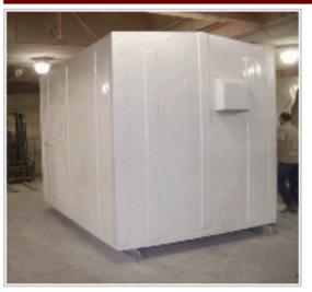
This fully insulated 8 x 12 fiberglass communication shelter was fabricated by VPC for the US Coast Guard for their communication equipment. This building was built with Radio Frequency Interference (RFI) shielding to protect the equipment stored inside. The floor is reinforced with a steel skid and is outfitted with heat, a/c, exhaust and mounting options. Fiberglass is an ideal composite material in conditions where salty sea spray and extreme weather conditions exist
