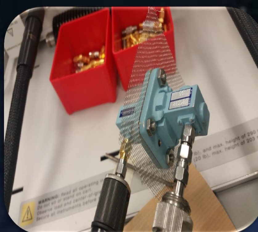
(Above) PNA Network Analyzer test setup (Below) 18 Mesh inside Waveguide Analyzer
