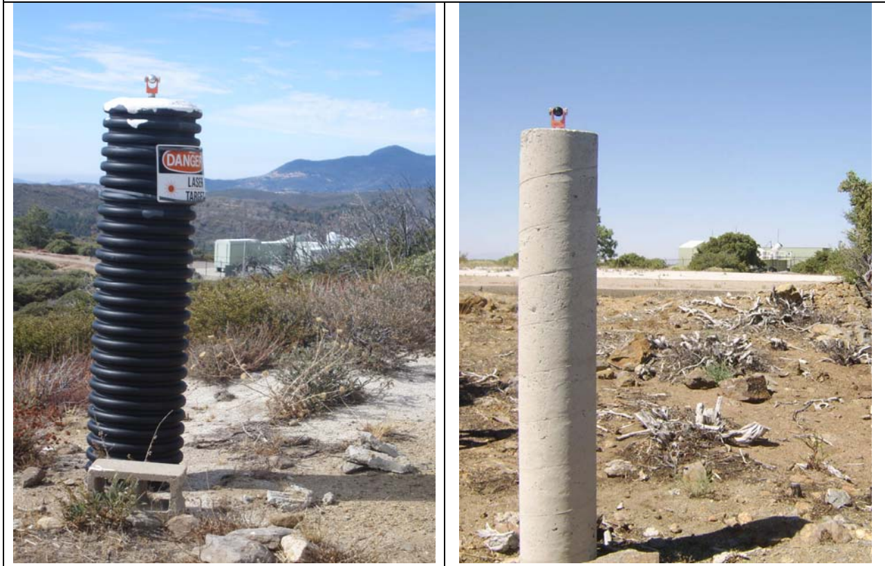
Calibration Piers to MOBLAS-4
